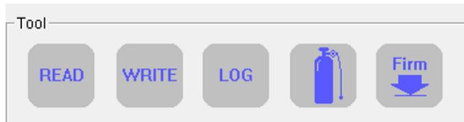
**READ:** By pressing the “Read” it displays current settings of the SGT/SGT-P and will discard any unsaved changes in the Tab.
